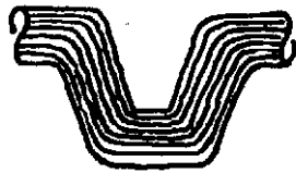
Forging True grain flow
