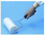
60 sheets of 14-in. length. While the Foam type Roller Refill provides 20 sheets of 16-in. length. Both sheets are perforated at circumferential distances, and the Film Type Refill has an uncoated edge. When a sheet becomes contaminated it is simply peeled off to clean it. When the Refill is used up, it is slid off the Handle and a new Refill simply slides on.
