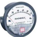
*Housing:* Die cast aluminum case and bezel, with acrylic cover. Exterior finish is coated gray to withstand 168 hour salt spray corrosion test.
