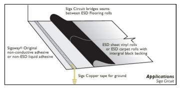
ESD roll flooring with fully conductive backings are then installed over the **Sigaway®** with **Siga Circuit** adhesive. 8" wide tape is frequently used to electrically bridge loose lay matting head to head or side to side
