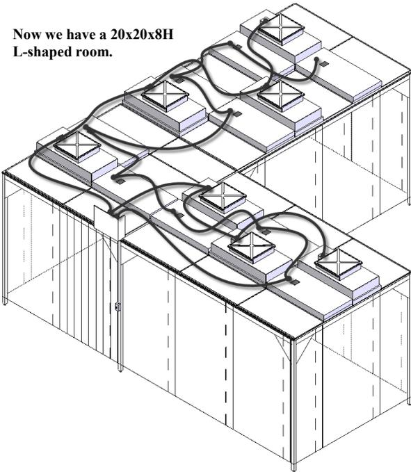
Once again we were able to use the curtains from one wall of the original 8x8x8H room on the end of the new addition. Also we were able to add the filters and lights to the existing Prefab Wiring Kit.
