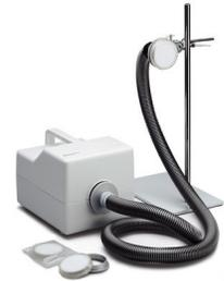
When the virus concentration is to be determined, the gelatin filter must be dissolved after sampling, so that retained viruses can be cultivated in the solution and analyzed by virological or molecular biological methods.
